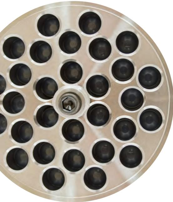
The CECO rMAX™ high-speed valve is engineered to withstand harsh field operating conditions. CECO's unique valve design allows rMAX™ to last longer even in dirty and wet gas applications. Contoured valve seats and specially-designed poppet heads minimize liquid or debris entrapment that can cause early failure in disc and ported plate valves. The result is longer compressor run times and less frequent valve replacement, allowing greater gas throughput and dramatic costs savings.
